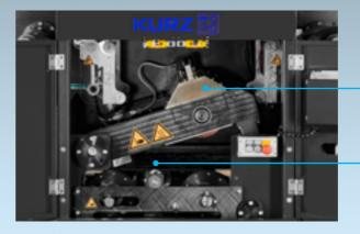
**High quality metallisation** – accurate temperature and quick warm up time using an infrared heating system in combination with a silicone stamping wheel
