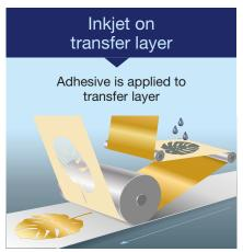
The heart of our inkjet on transfer layer technology is the innovative inkjet technology combined with the KURZ DIGITAL METAL® finishing solution. Experience digital metallization and create optimal finishing results with high-gloss, flat metallic effects and deep color brilliance.
