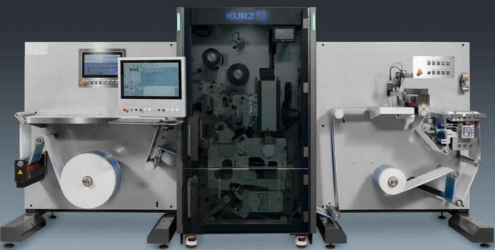
Thanks to the unique 'inkjet on transfer layer' technology of the DM-UNILINER 2D, the surface to be printed remains unchanged, despite the large number of possible substrates. This makes it easy to achieve highly variable finishing. For you, this means full control of the processes with less effort since no in-depth inkjet printing knowledge is required to finish with consistently high quality.
